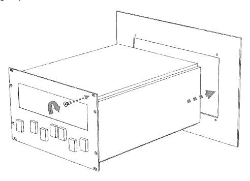
**Note:** the circulation of cooling air on the upper and bottom side and behind the device must not be significantly limited when the unit is inserted in a rack or laid on a table.
