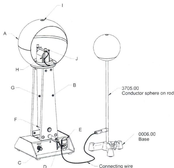
The band generator is used to produce very high DC voltages with low amperage, which makes experiments with the generator harmless.
