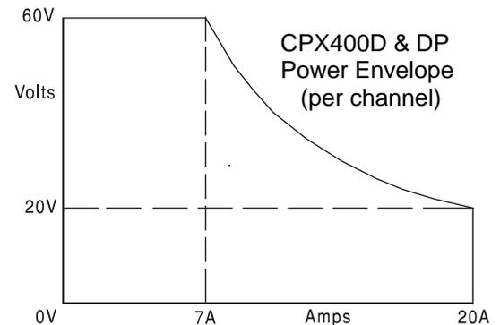
Operating Ranges: Four selectable ranges: 60V/20A, 60V/7A, 20V/20A and Custom Limits.
