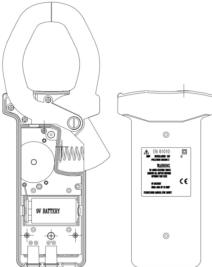
When the low battery symbol is displayed on the LCD, replace the old battery with a new battery.
