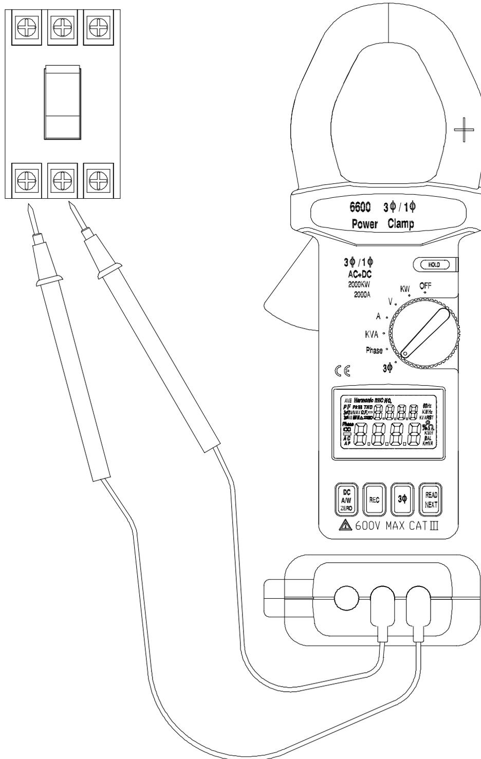
**WARNING:** Maximum input for DC V is 1000, and for AC V is 750. Do not attempt to take any voltage measurement that exceeds these limits. Exceeding these limits could cause electrical shock and damage to the clamp meter.
