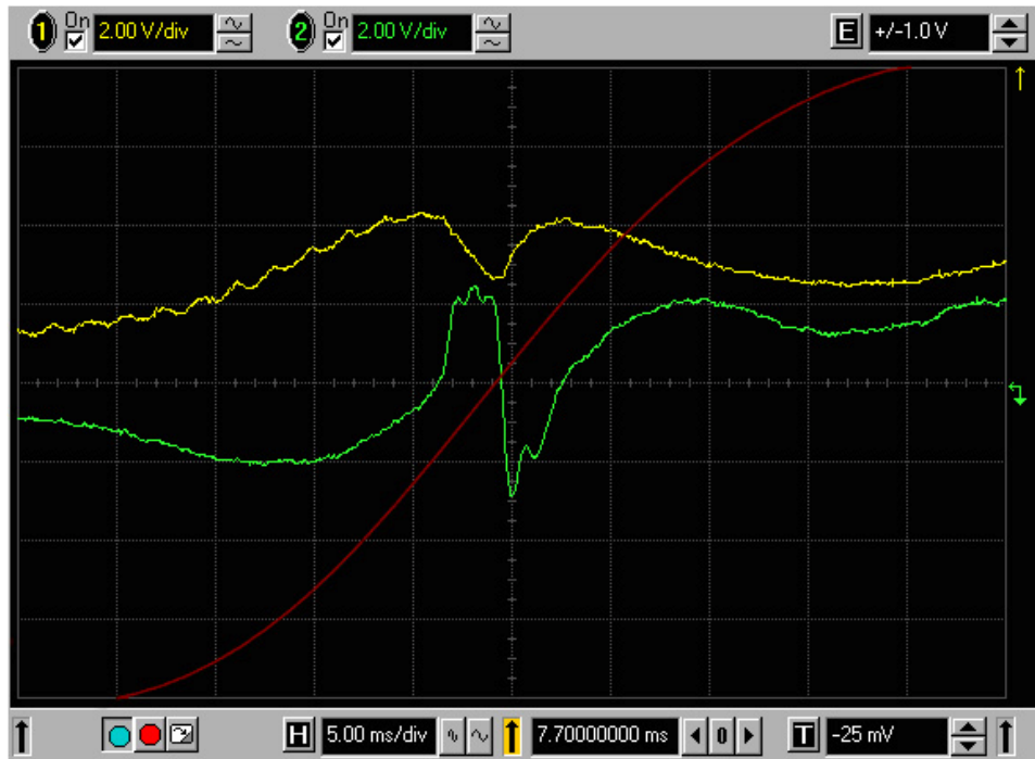
Figure 4. Image of correctly adjusted spectroscopy signals. Yellow line is the spectroscopy absorption signal from the photodiode, green line is derivative signal form the Lock-In Amplifier and red line is PZT scanning voltage from the Sinus Generator. Slope of the green line in the center of the screen has to be adjusted to be maximally steep with midpoint at zero crossing.
