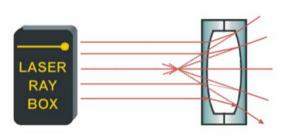
E19b Light beam passing through air convex lens – the rays are non-parallel to the optical axis (RODS+)
