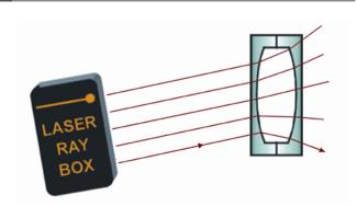
E20a Light beam passing through air concave lens – the rays are parallel to the optical axis (RODS+)
