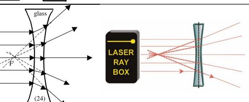
E18b Light beam passing through glass concave lens – the rays are non-parallel to the optical axis (RODS/RODS+)
