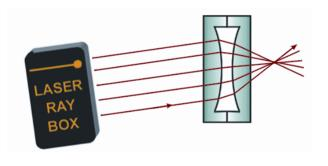
E21a Parameters of thick lenses - determination of radius of curvature (RODS/RODS+)
