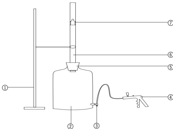
The precision tube is used together with the Marriott bottle U14327 to determine the adiabatic exponent  $c_p/c_v$  using Rüchardt's method.
