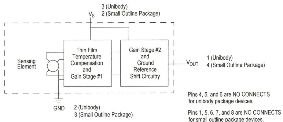
**Figure 1. Fully Integrated Pressure Sensor Schematic
