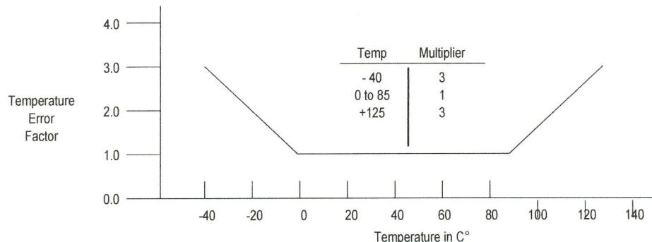
NOTE: The Temperature Multiplier is a linear response from 0x to -40°C and from 85° to 125°C.
