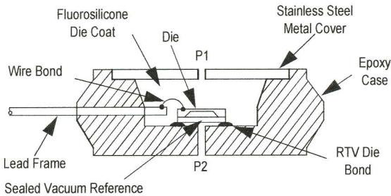
Figure 2. Cross Sectional Diagram (not to scale)
