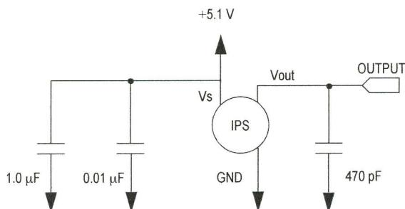
Figure 3. Recommended Power Supply Decoupling and Output Filtering
