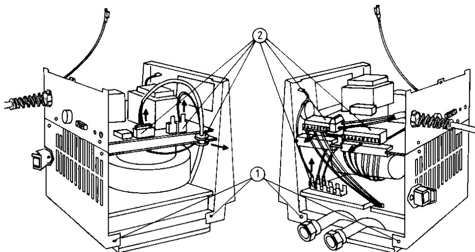
There is no provision for a fuse for the complete unit since the necessary 16A fuse corresponds to the mains fuse usually provided at the location. The control circuit of the unit has a separate fuse; a fuse 5 x 20 F4A is located in the control unit. This is accessible after removing the cover. When the fuse has blown the green lamp in the mains switch does not light up.
