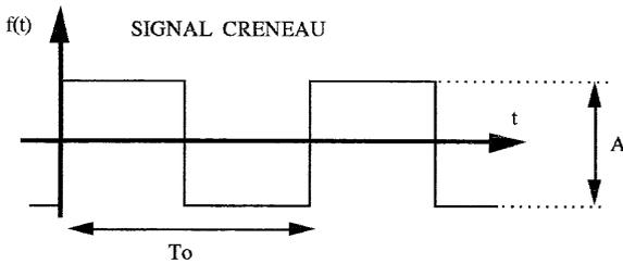
$$f(t) = 0 + \left[ \frac{2A}{\pi} \cdot \left[ \sin \omega_0 t + \frac{\sin 3\omega_0 t}{3} + \frac{\sin 5\omega_0 t}{5} + \dots + \frac{\sin (2n+1)\omega_0 t}{(2n+1)} + \dots \right] \right]$$
