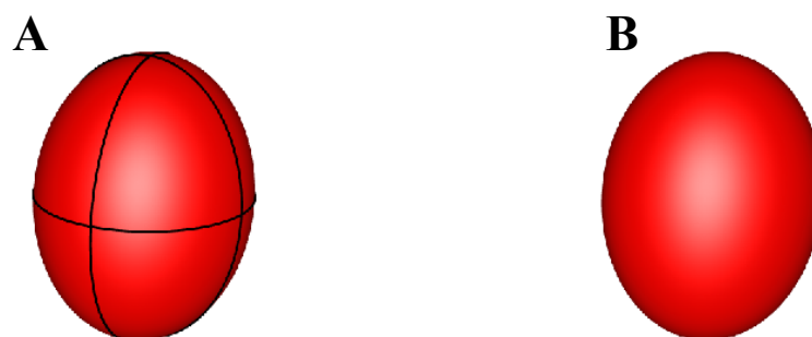
Figure 12.3: Displacement ellipsoids of an atom (A) with principal ellipses and (B) without them.
