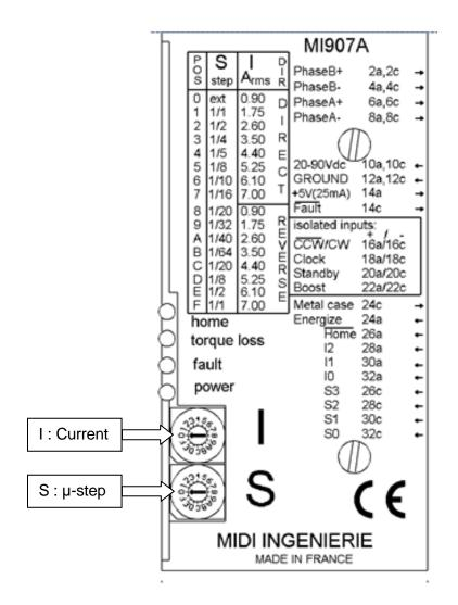
Format 3U : 100 x 160 x 54 Connector : DIN 41612, 32 pins type D
