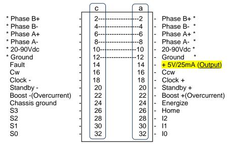
Be careful! Regarding the pin N° 14a, it is a voltage output 5V/25 mA made for polarization of the opto-isolated inputs. Don't connect with any external power.
