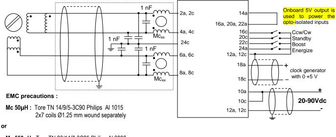
Mc 550µH : Tore TN 23/14/7-3C25 Philips Al 3800 2x12 coils Ø2.25 mm wound separately and
