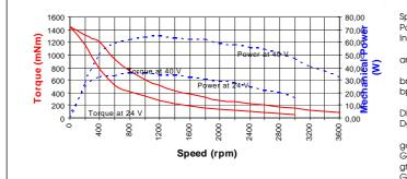
The above statements are given for a 100% value of the setpoint torque and for two supply voltage values (24 and 40 VDC).
