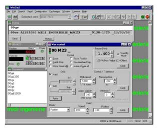
**WINSIM2** is a software-based Human Machine Interface allowing easy communication with one or several modules (SIMPA, MAC and DMAC family) from a Windows PC.
