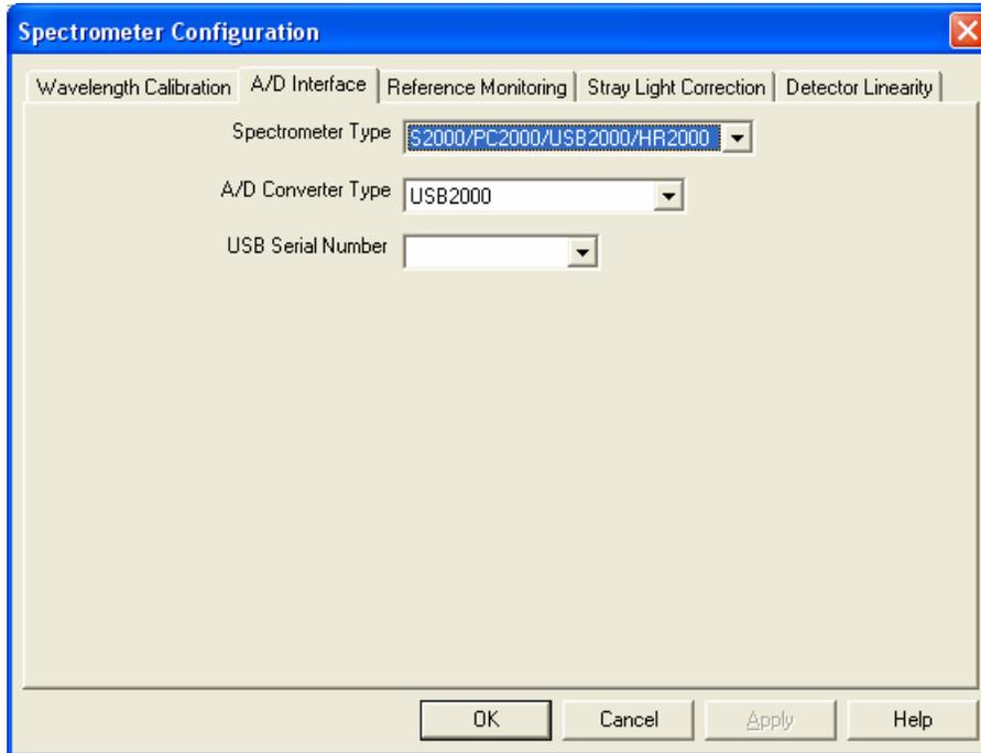
5. On the **A/D Interface** tab, enter the same values that you entered in the **Configure Hardware** screen (see [Configure Hardware Screen](#)). When you exit the OOIBase32 application, this data is stored in the .SPEC file.
