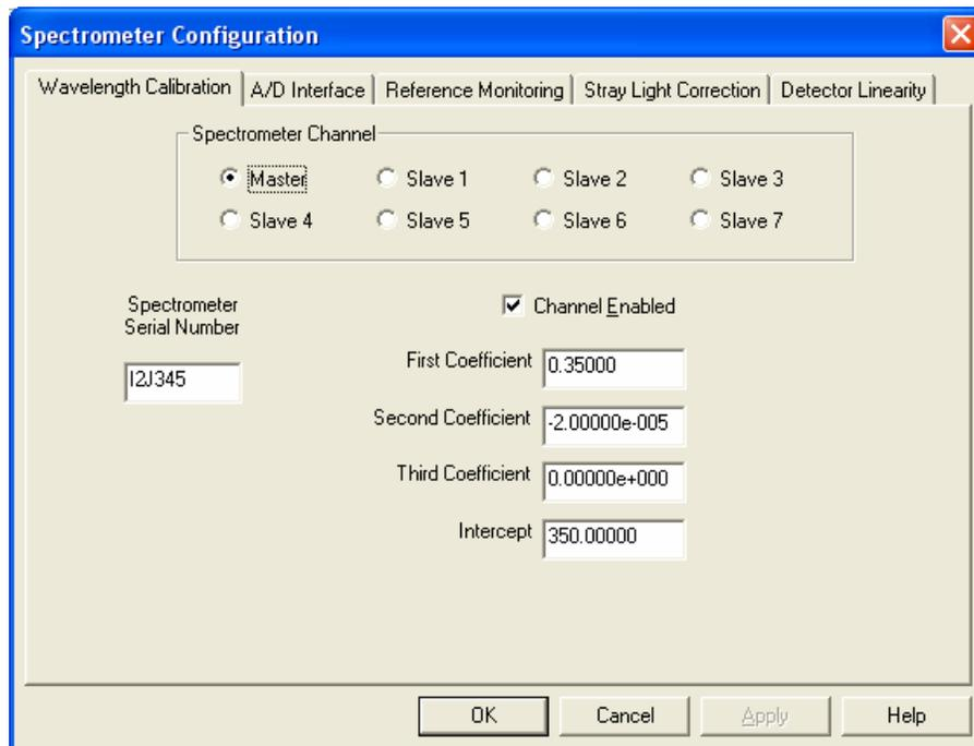
2. On the **Wavelength Calibration** tab, ensure that the calibration coefficients (read from a memory chip in the Curie spectrometer) match the coefficients listed on the Wavelength Calibration data sheet that came with your spectrometer.
