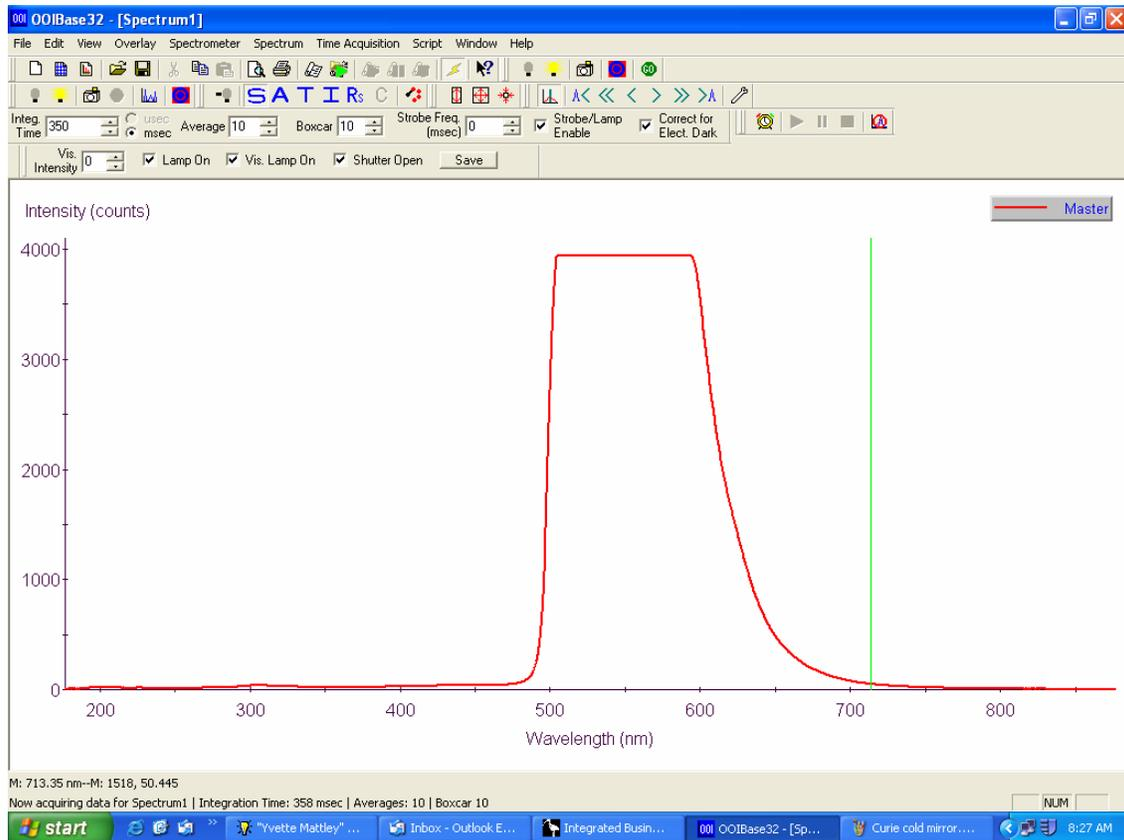
**Saturated Fluorescein Signal in Scope Mode**
