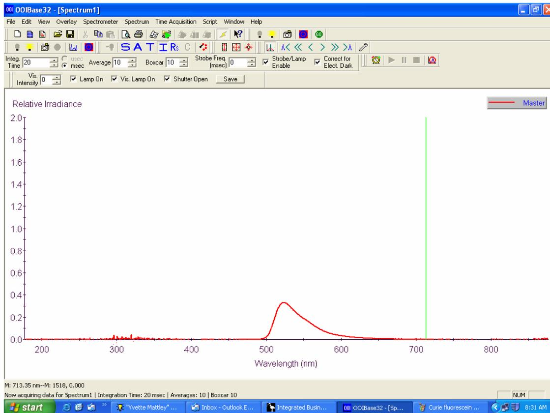
**Unsaturated Fluorescein Signal in Relative Irradiance Mode**
