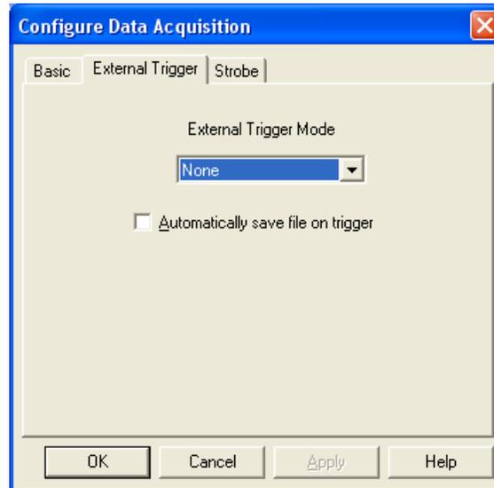
3. In the **External Trigger Mode** field, select **None** to disable the pushbutton, and click **OK**.
