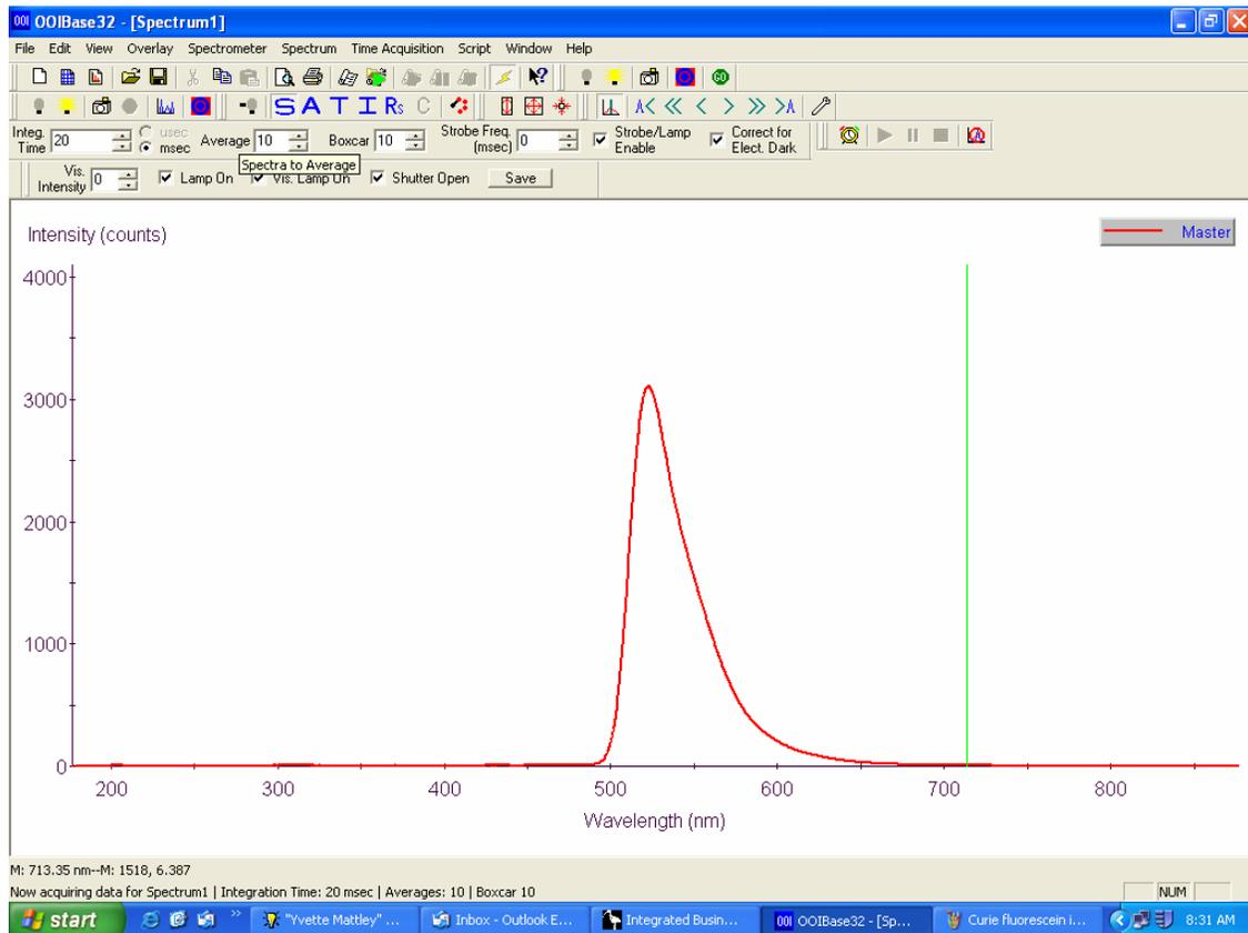
**Unsaturated Fluorescein Signal in Scope Mode**
