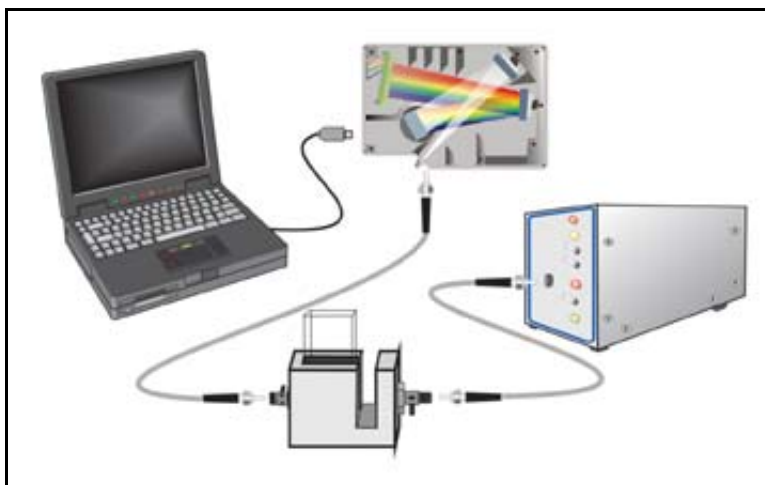
Figure 6-1: Typical absorbance setup. The light source (far right) sends light via an input fiber into a cuvette in a cuvette holder (bottom center). The light interacts with the sample. The output fiber carries light from the sample to the spectrometer (top center), which is connected to the PC (far left).
