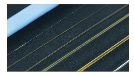
The FT-KIT Fiber Tinkerer Kit (left) includes an assortment of randomly selected, unterminated UV-VIS and VIS-NIR optical fibers. Each fiber included in the kit will be at least 1 meter in length. The Fiber Termination Kit (TERM-KIT) on the following page includes all the tools needed to terminate and polish fiber.
