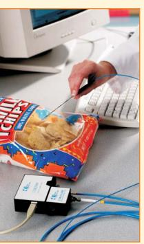
Optical sensors can be used for a variety of applications. Here, our FOXY Fiber Optic Oxygen Sensor monitors headspace gases in food packaging.
