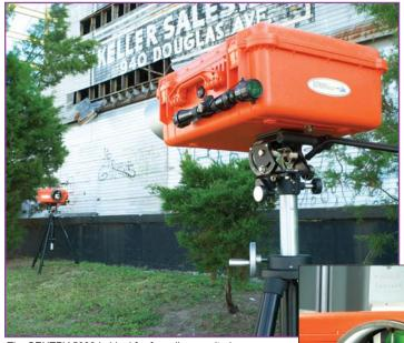
The SENTRY-5000 is ideal for fenceline monitoring applications of up to 850 meters. The SENTRY-STAN (at right, being inserted into the optical path of the SENTRY-5000) is a NIST-traceable calibration cell that comes with the SENTRY-5000.
