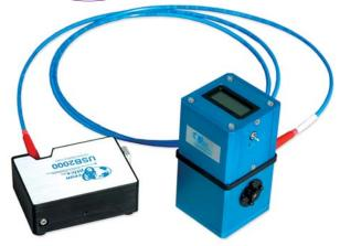
In this setup, the LED-PS is on top of the FOIS-1 Integrating Sphere and a P400-2-VIS-NIR Optical Fiber collects the light energy from the FOIS-1 and sends it to the USB2000 Spectrometer. Our software reports the absolute spectral intensities for the LED as well as color values, photopic data and more.
