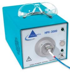
The HPX-2000 Xenon Light Source (185-2000 nm) is especially useful for fluorescence applications, and for other applications where a high-intensity lamp is necessary. The HPX-2000 has an integrated shutter, which can be driven either by a switch or by a TTL signal. It also comes equipped with a slot for filters up to 25-mm diameter or square, and up to 14-mm thick. (If operating the HPX-2000 for ultraviolet applications, use the solarization-resistant fiber described on pages 139-140.)
