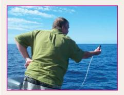
A USB2000 Spectrometer set from 360-1100 nm measures reflectance and irradiance. The USB2000 connects to a patch cord that screws into a Gershun Tube, which has fixtures for adjusting the area of light entering the fiber -- in this case, to reduce the field of view to 3°. Upwelling irradiance and downwelling radiance measurements -- the spectral distribution of the underwater light field -add valuable data.
