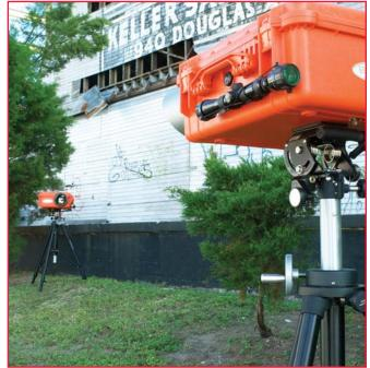
CEREX Environmental Services, Inc. is an OEM that uses one of our highresolution spectrometers in its Sentry and Hound Monitoring Systems, advanced, EPA-approved detection methods for conducting real-time partsper-trillion analysis of toxins in the air. See pages 24-25 for details.
