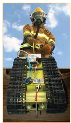
American Standard Robotics in St. Petersburg, Fla., prepares one of their VGTV-Xtreme Reconnaissance Vehicle robots equipped with an Ocean Optics spectrometer to identify the chemical involved in a simulated hazardous-material tanker trailer.
