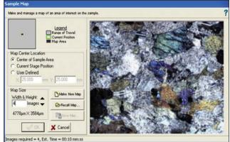
View an exact spot of the sample before, during and after the ablation process. The LIBS-ELITE provides real-time, high-resolution qualitative analysis of trace elements in diverse materials such as metals, biological tissues, soils, optics, semiconductors, gems, and other geological, biological and environmental specimens.
