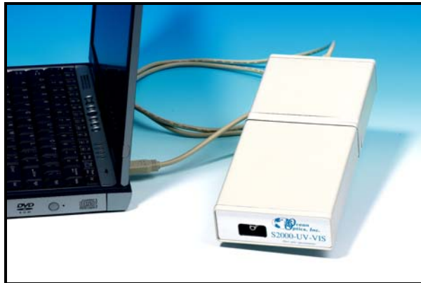
The ADC1000-USB connects to the back of an S2000 Spectrometer and interfaces to a notebook computer via the USB port and USB cable.
