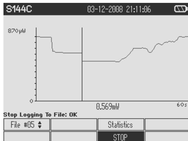
After pressing the START button the data that are sampled in these screens will be stored to the built in SD memory card on the selected file until STOP is pressed. With START the selected file will be overwritten.
