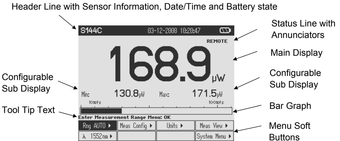
Figure 5 Numeric Display Setup
