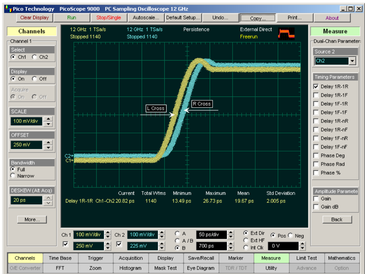
Two waveforms with entered deskew of 20 ps
