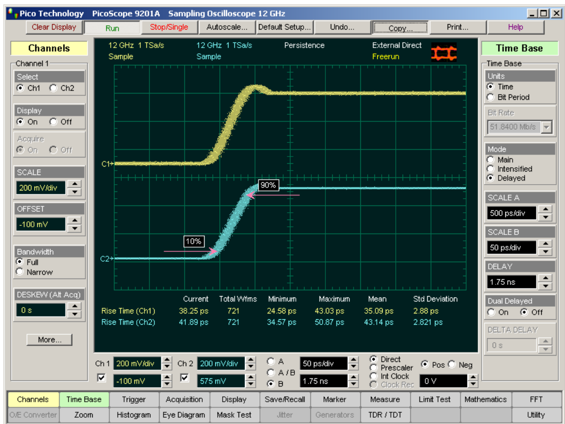
Channel 1 (yellow trace): full bandwidth 12 GHz Channel 2 (blue trace): narrow bandwidth 8 GHz
