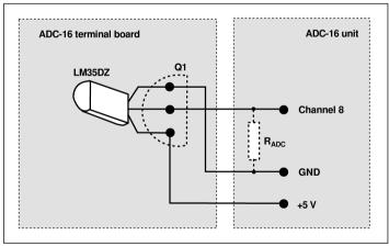
Temperature sensor circuit with LM35 IC
