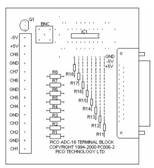
Layout of ADC-16 Terminal Board
