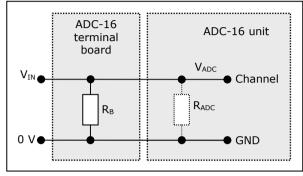
Shunt resistor circuit
