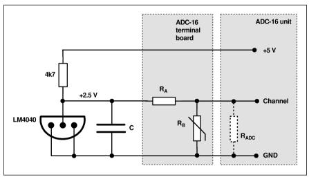
Temperature sensor circuit with precision thermistor
