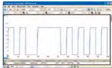
Crank sensor (Hall effect)
