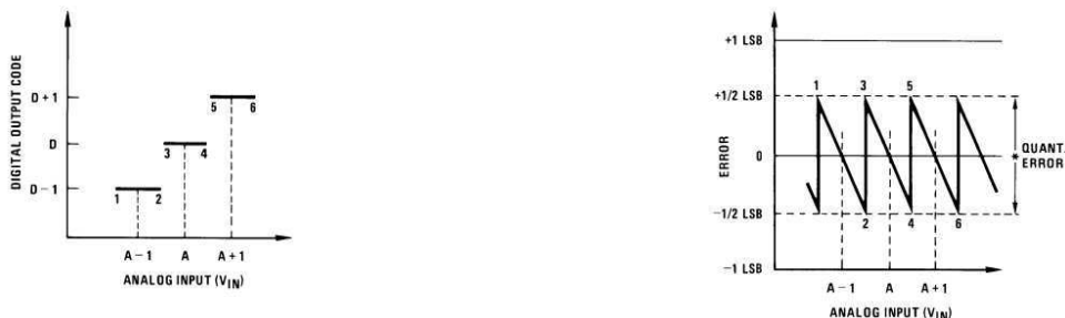
Figure 45. Clarifying the Error Specs of an A/D Converter Accuracy = \pm 0 LSB: A Perfect A/D
