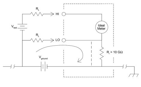
$R_L$  = Lead Resistance  $R_i$  = Multimeter Isolation Resistance  $V_{ground}$  = Voltage Drop on Ground Bus
