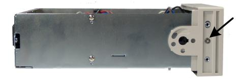
7 Remove the two screws holding the front panel.
