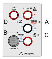
**Note:** The front-panel terminals and current protection fuse are shown above.
