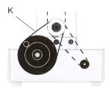
If you want to drive the belt manually, the drive belt (K) is moved from the pulley on the motor, to the crank pulley instead.
