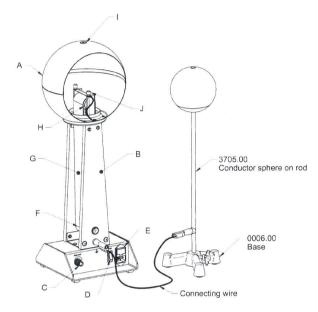
The band generator is used to produce very high DC voltages with low amperage, which makes experiments with the generator harmless.
